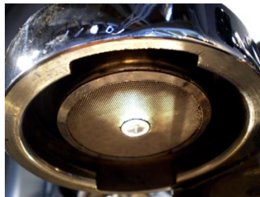
Diffusion Screen Inside the Group Head
