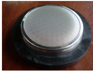
Head Seal and Diffusion Screen
