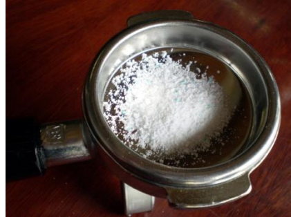
Blind Bucket Loaded with Powder
